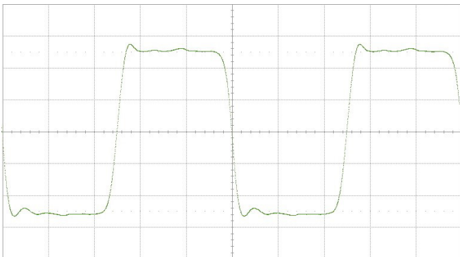
Fig. 11: 2 GHz RF Output @ P_{IN} = -8 dBm (sinewave) 2 V/div
